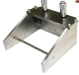
The applicator is specially designed for research and development purpose with user variable coating thickness using micrometer, adjustment from 0- 10mm in steps of 10 microns.
