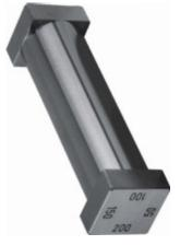
Combining four gaps sizes in one unit. Provides excellent results on firm and smooth substrates. By simply rotating through 90\*, the next gap size is placed on the test surface.
